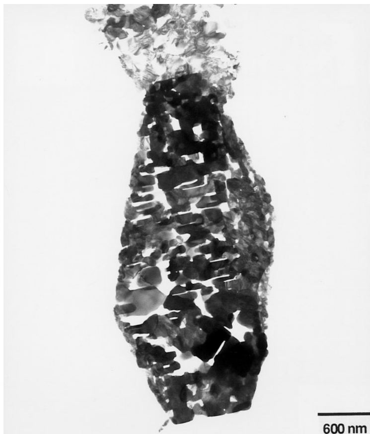
FIG. 11. Bright field image of a precursor particle calcined at 800°C under nitrogen for 24 h.
